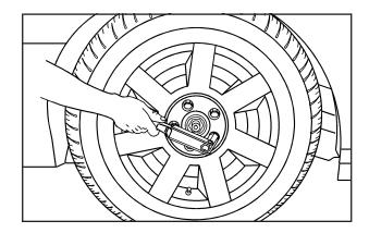
3. For models with exposed lug nuts, loosen them using the wheel wrench. Do not remove them yet.
